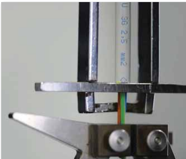
A sample in the stripping test.
