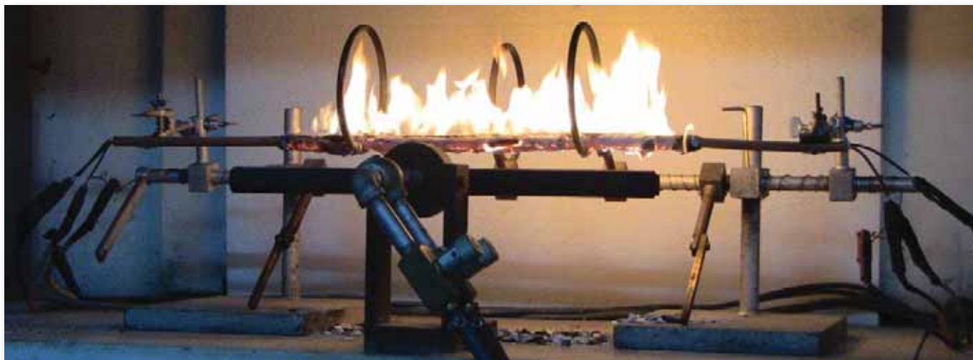
A cable samples in the test for burning under voltage.
