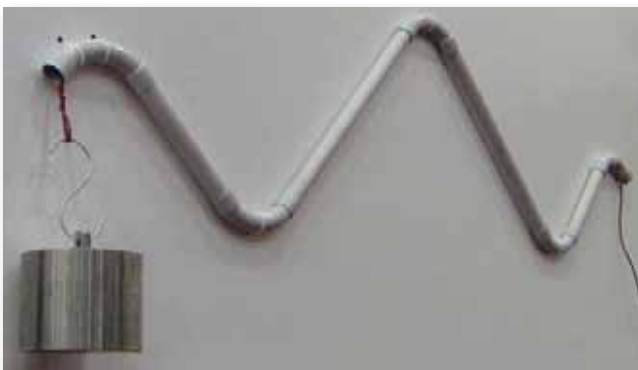
A cable sample in the slickness test.
