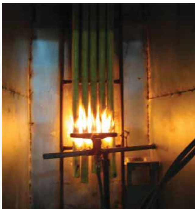
Cable samples in the harnessed cable burning test.
