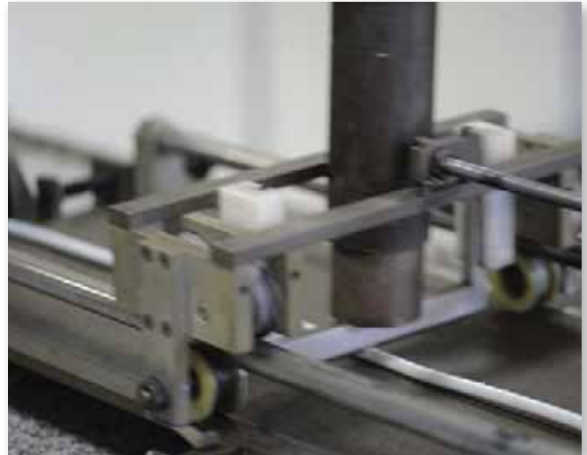
A cable sample in the abrasion test.
