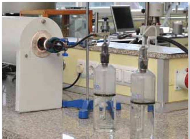
The halogen amount is measured by absorption of the burning gas into water.
