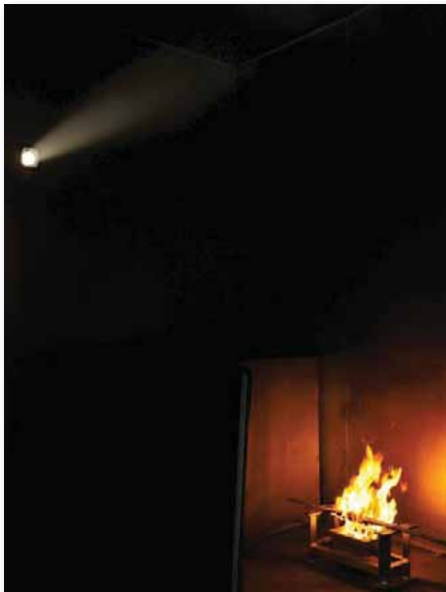
A cable sample in the smoke density test.
